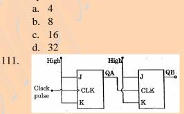
The above circuit illustrates a typical application of the JK flip-flops. What does this represent?
