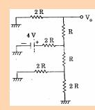
What is the output voltage ' $V_0$ ' of the R-2R decoder ladder network?
