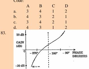
The gain-phase plot of a linear control system is shown in the above figure.
