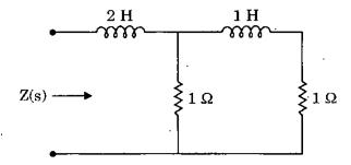
Consider the above network. Impedance of this network as a function of the complex frequency s consists of a certain number of zeros and poles. What is the location of poles?
