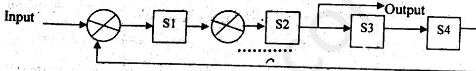
This pipeline has a total evaluation time of six clock cycles. All successor stages must be used after each clock cycle.
