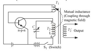
In an oscillator, a sustained A.C. output is obtained without any input oscillation. For this to happen, the output of a transistor amplifier is fed back into its input. This is achieved by coupling the winding  $T_1$  to winding  $T_2$ .
