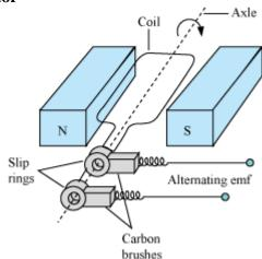
An A.C. generator consists of a rotor shaft on which a coil is mounted. A magnetic field is created around an armature coil with the help of permanent magnets.
