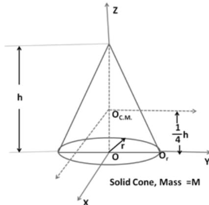
then the moment of inertia about another axis parallel to the X axis, but passing through the point  $O_r$  (see figure), is
