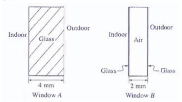
Window A is a simple pane of glass, 4 mm thick. Window B, on the other hand, consists of two extremely thin panes of glass, separated by an air gap of 2 mm, as shown in the figure above. If the thermal conductivity of glass is known to be 0.8 Wm-1K-1 and that of air is 0.025 Wm-1K-1, then the ratio of heat flow  $Q_A$  through Window A to the heat flow  $Q_B$  through Window B is given by
