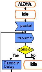
Figure: Description of terminal behavior in ALOHA random access network
