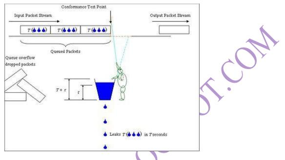
Figure 3: Traffic shaping with a leaky bucket as a meter
