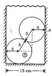
In the figure shown, consider the two identical spheres with radius 5 cm, weight 100 N each and the distance between the two walls as 15 cm. What is the reaction force at point A?
