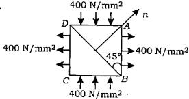
The square element in the figure is subjected to a biaxial stress of  $400 \text{ N/mm}^2$  as shown. What is the intensity of normal stress  $p_n$  on the plane BD?
