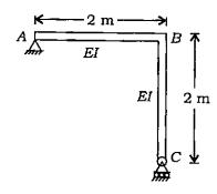
What is the force required for displacing support C horizontally through a distance  $\Delta$ ?
