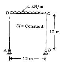
What is the bending moment at *B* for the symmetrical portal frame shown, which is subjected to a uniformly distributed load of 1 kN/m on the beam portion?
