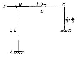
In the portal frame shown, find the ratio of moments  $M_{BA}$  and  $M_{CD}$  induced at the column heads due to sidesway
