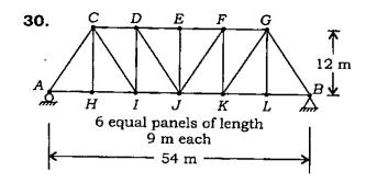
For the pin-jointed plane truss shown in the figure, which of the following diagrams represents the influence line for the bar force in the member DI, when a load travels on the bottom chord?
