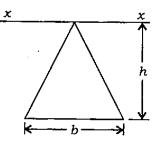
What is the moment of inertia of the triangle with respect to xx as shown in the figure?
