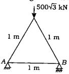
(Cross-sectional area of each member  $\approx 50 \text{ mm}^2$ , modulus of elasticity  $E = 2 \times 10^5 \text{ N/mm}^2$ )
