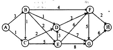
The distance (in miles) between different stations is shown on each link. Determine the shortest route from station A to station 4.
