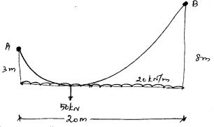
IX. Draw bending moment diagram for the three hinged parabolic arch shown in figure.
