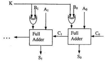
If the operands are in 2's complement representation, which of the following operations can be performed by suitably setting the control lines K and C o only (+ and -denote addition and subtraction respectively)?
