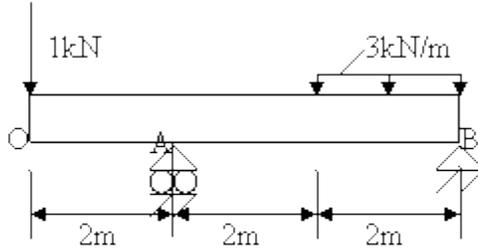
A beam is supported and loaded as shown in Fig.6. Draw the S.F. and B.M. diagrams. Find the maximum bending moment and its location. **(14)**
