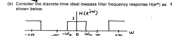
Impulse response and frequency response of an LTI system are a fourier transform pair. Determine and sketch impulse response of the ideal LPF from the frequency response shown.
