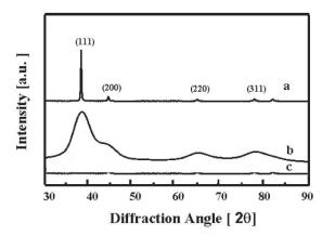
(along with lattice planes) and (b) nanoparticles of gold that were synthesized in a research lab. These were deposited on the same flat polymeric substrate and (c) is a blank polymeric substrate.
