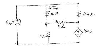
12. (a) (i) Find  $i_0$  in the following circuit using superposition. (10)
