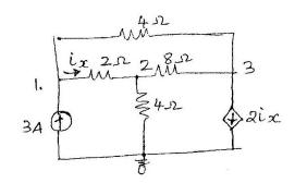
(ii) Use mesh analysis to find the current  $I_0$  in the following circuit: (8)
