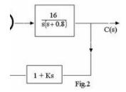
Determine the values of K such that the damping ratio  $\xi$  is 0.5. Then obtain the rise time  $t_r$ , peak time  $t_p$ , the maximum overshoot  $M_p$  and settling time  $t_s$  from the unit-step response. (16)
