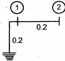
In the network as shown above, the marked parameters are p.u. impedances. The bus-admittance matrix of the network is
