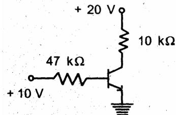
In the transistor circuit as shown above, the collector to ground voltage is + 20 V. The possible condition is
