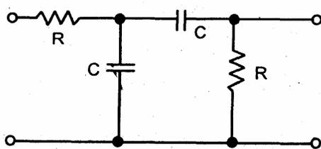
An FET oscillator uses the given phase shift network as shown above. The minimum gain required for oscillation is
