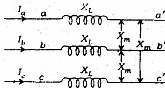
The above circuit shows a 3-phase system having a balanced self-inductive reactance of  $X_L$  per phase a mutual reactance of  $X_m$  between pairs of phases. The line currents are  $I_a$ ,  $I_b$  and  $I_c$ , and they may be unbalanced.
