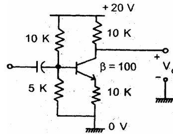
Consider a silicon transistor connected as a common emitter amplifier as shown above. The quiescent collector voltage of the circuit is approximately
