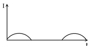
Sol: Diode acts as a half wave rectifier without filter.
