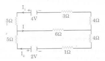
In the given circuit, calculate (i) value of  $I_1$ , (ii) value of  $I_2$  and (iii) terminal voltage at the cell of e.m.f. 4 volt (iv) current in  $6\Omega$  wire :
