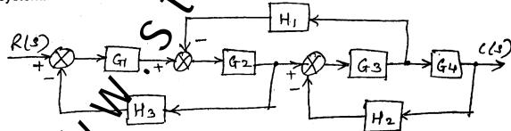
(b) Consider the following block diagram shown. Draw its equivalent signal flowgraph 10 and fine the transfer function  $\frac{C(s)}{R(s)}$  using Mason's Gain Rule.
