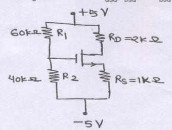
$V_{TN} = 1 V$   $K_n = 0.5 \text{ mA/V}^2$
