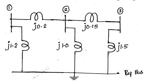
13. Carry out one iteration of power flow analysis for the power system with the following data and given the voltages in polar form at the end of I iteration by NR method.
