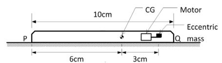
Given in addition that the eccentric mass = 2 grams, eccentricity = 2.19 mm, mass of the mobile = 90 grams, g = 9.81 m/s<sup>2</sup>. Uniform speed of the motor in RPM for which the mobile will get just lifted off the ground at the end Q is approximately
