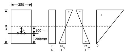
Since the tensile stress at bottom face of the beam is zero,
