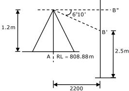
True staff reading at station B =  $2.5 - 0.0673 \times 2.2^2 = 2.174 \text{ m}$ Now, B'B" =  $(\tan 6^{\circ} 10^{\circ}) \times 2200 = 237.701 \text{ m}$
