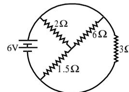
46. The total current supplied to the circuit by the battery is:
