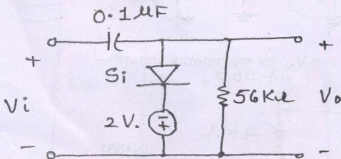
For the given network find  $V_o$  of the circuit, compare it with half the period of applied signal and sketch  $V_o$  if  $V_i$  is 20 V P-P, square wave, 1 kHz waveform.
