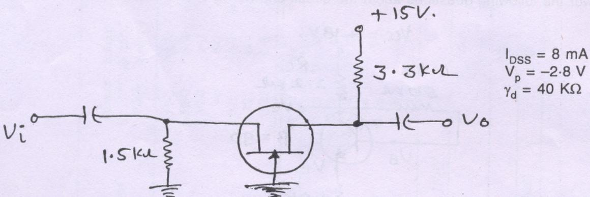
4. Design a single stage CS JFET amplifier using Potential Divider Biasing for the following specifications :— 20
