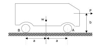
2.14. A simply supported beam carries a load 'P' through a bracket, as shown in Fig.2.14. The maximum bending moment in the beam is
