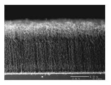
Carbon nanotube "shag electrode" in ultra-capacitors for energy storage (MIT)
