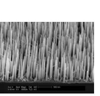
Vertical growth of nanowires for electronic devices (Stanford)
