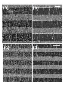
Electric field aligning of nanowires (U. Mass)
