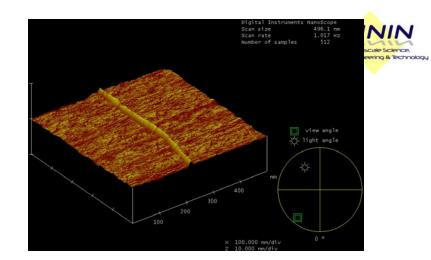
AFM image of carbon nanotube
