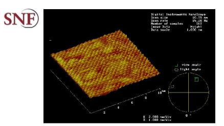
AFM image of mineral surface showing atomic structure.
