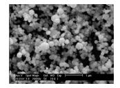
Nanoparticles by flame pyrolysis (Princeton)
