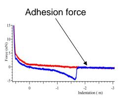
AFM force measurements of the tip interaction with the bilayer.
