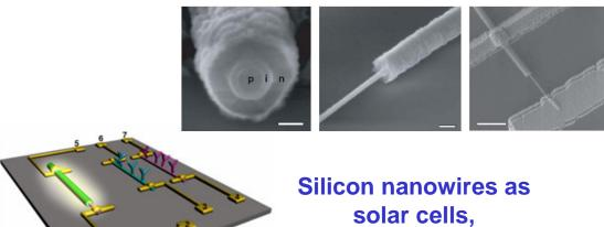
solar cells, nanoelectronic power sources, and sensors (Stanford)
