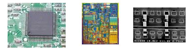
• Makes use of depositing thin films, then "photolithography" and plasma etching to make films into desired patterns on a silicon wafer.
