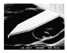
AFM tip, used to manipulate, image and measure atomic scale features.
