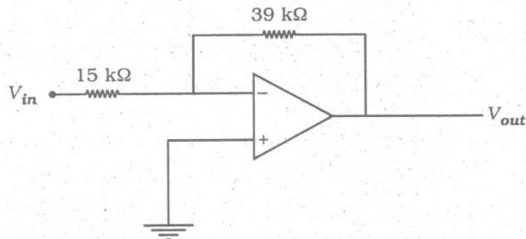
Find the output of the ideal operational amplifier shown in the following figure for the input of  $V_{in} = 120 \text{ mV d.c.}$
