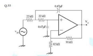
For the given low-pass circuit shown in the figure, the cutoff frequency in Hz will be
