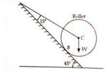
b. A roller of 850 N is resting on a smooth inclined plane and is held by a string as shown in Fig.1. Determine the (i) reaction at B (ii) tension in the string. (10)
