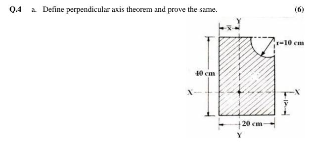
b. Locate the centroid of the shaded area shown in Fig.3.
