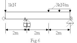
beam is supported and loaded as shown in Fig.6. Draw the S.F. and B.M. diagrams. Find the maximum bending moment and its location. (14)
