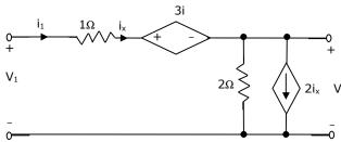
11. Find the current transfer-ratio,  $\frac{I_2}{I_1}$ , for the network shown below (figure). Also, mark all branch currents
