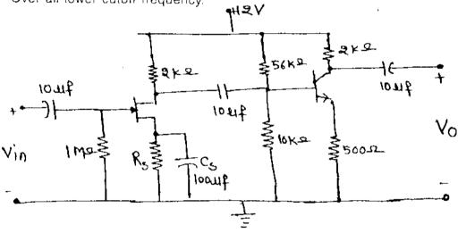
Design a two stage R-C coupled BJT amplifier using BJT BC 147A for the following requirement 20
