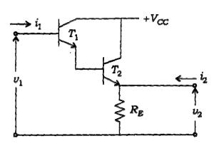
For the Darlington amplifier shown in figure above, obtain its Z-matrix for identical  $T_1$  and  $T_2$  having  $h_{fe} = 100$ ,  $R_E = h_{ie} = 1$  k
