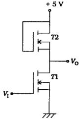
$$\begin{split} r_{d(ON)} & \text{for } T2 = 100 \text{ k}\Omega \\ r_{d(OFF)} & \text{for } T2 = 10^5 \text{ M}\Omega \\ r_{d(ON)} & \text{for } T1 = 1\Omega \\ r_{d(OFF)} & \text{for } T1 = 10^4 \text{ M}\Omega \\ \end{split}$$
