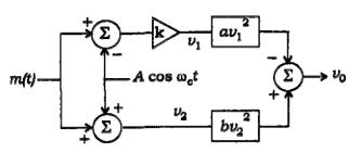
What would be the value of gain k in figure above to yield the suppressed carried DSB signal?
