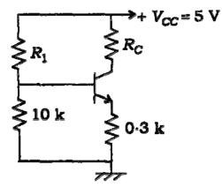
The BJT in amplifier of figure above has  $h_{fe} = 100$ ,  $V_{BE} = 0.7V$ ,  $I_{CO} = 0$ . Calculate the values of  $R_1$  and  $R_C$  such that its  $I_C = 1$  mA and  $V_{CE} = 2.5$  V.
