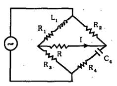
In the circuit shown above when I = 0, show that  $\omega L_1/R_1 = 1\omega C_4R_4$ .
