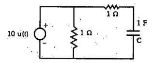
In the circuit shown above, determine the initial and final values of the current through the 1 F-capacitor. Make use of theorems.
