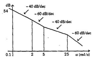
From the asymptotic approximation plot of dB versus  $\omega$  of a minimum phase system with real poles and zero shown in the above figure, determine the poles and zero of the system
