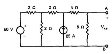
Find  $V_{AB}$  for the circuit shown above using source transformation.
