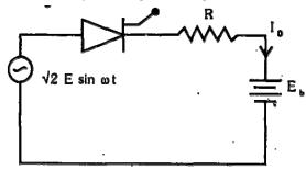
Derive an expression for the average charging current in terms of source voltage E, back e.m.f. and resistance R. The SCR is fired continuously. If E = 220 V (r.m.s.),  $E_b = 100 \text{ (DC)}$  and R = 10 ohms, calculate —
