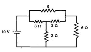
Determine the value of H shown in the above figure such that the 6  $\Omega$ -resistor consumes the maximum power.
