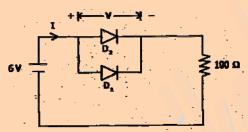
In the given circuit,  $D_1$  is an ideal germanium diode and  $D_2$  is a silicon diode. having its cut-in voltage s 0.7V, forward resistance as  $20\Omega$  and reverse saturation current ('s) as 10 nA. What are the values of I and V for this circuit, respectively?
