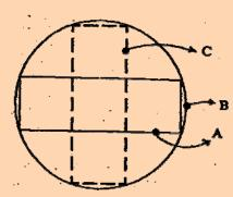
A rectangular waveguide (A) is gradually deformed first into a circular waveguide (B) and back again into a rectangular waveguide (C) which is oriented through  $90^{\circ}$  with respect to (A). If the input mode is  $TE_{10}$ , which mode is excited in the output waveguide (C)?
