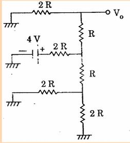
What is the output voltage ' $V_o$ ' of the R-2R decoder ladder network?
