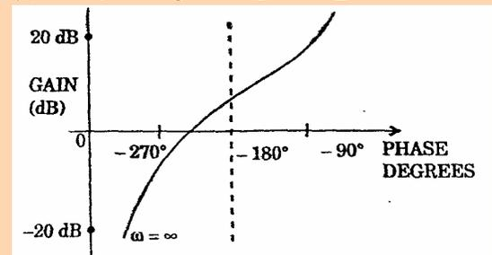
The gain-phase plot of a linear control system is shown in the above figure.
