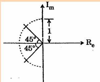
A diaphragm type pressure sensor has two poles as shown in the figure above. The zeros are at infinity. What is its steady state deformation for a unit step input pressure?
