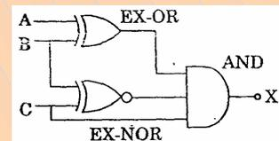
For the logic circuit shown in the above figure, what is the required input condition (A, B, C) to make output X = 1?
