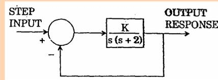
A closed loop system is shown in the above figure.
