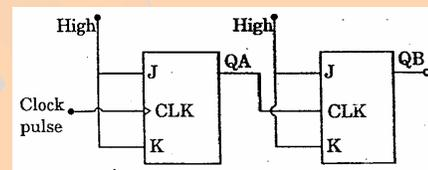
The above circuit illustrates a typical application of the JK flip-flops. What does this represent?
