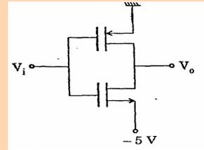
The threshold voltage for each transistor in the figure shown above is 20 V. What are the values of  $V_i$  for this circuit to work as an inverter?
