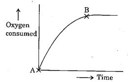
The above figure shows B.O.D. curve when the experiment was conducted at 20° C. If the experiment is conducted at 30° C, then the portion AB of the curve
