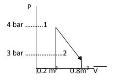
vii)Calculate the heat transferred during the cycle shown in the figure given below.
