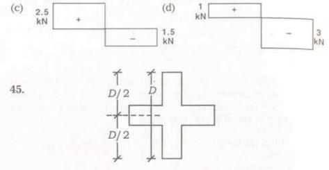
The cross-section of a beam in bending is as shown in the figure given above. It is subjected to a shear force acting in the plane of cross-section. Which among the following figures shows the correct shear stress distribution across the depth of the cross-section of the beam?
