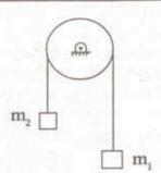
Two bodies of masses  $m_1$  and  $m_2$  are connected by a light inextensible string passing over a small smooth fixed pulley;  $m_1 > m_2$ . What is the acceleration of the system?
