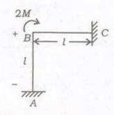
Members AB and BC in the figure shown above are identical. Due to a moment 2M applied at B, what is the value of axial force in the member AB?
