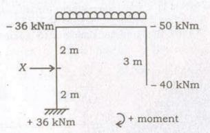
Final moment values got through the analysis of a portal frame have been shown in the figure given above. What is the value of X?
