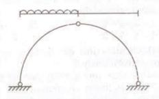
For the three-hinged parabolic arch shown above, which one among the following represents bending moment?
