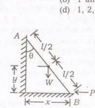
A ladder AB of weight W and length I is held in equilibrium by a horizontal force P as shown in the figure given above. Assuming the ladder to be idealized as a homogeneous rigid bar and the surfaces to be smooth, which one of the following is correct?
