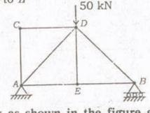
In a truss work as shown in the figure given abov what is the force induced in the member DE?
