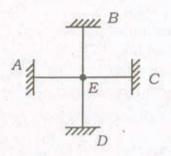
Four identical beams AE, BE, CE and DE have been rigidly jointed at E. The point C slips and rotates along with member firmly fixed at E. Which one of the following is correct?
