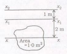
xx, x,x, and x,x, are parallel axes of which xx is the centroidal axis. If moment of inertia of the figure about x1x1 axis is 10 m4, what is the moment of inertia of the figure about x, x, axis?
