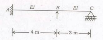
What are the distribution factors at joint B for the members BA and BC respectively, in the figure given above?
