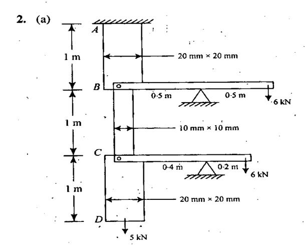
A stepped vertical steel bar ABCD is fixed at the top end A. Each segment of the bar AB, BC and CD is 1 m long and has cross-sections 20 mm  $\times$  20 mm, 10 mm  $\times$  10 mm and 20 mm  $\times$  20 mm respectively. A 5 kN load is applied directly at D and 6 kN loads are applied on the levers attached to the stepped bar at B and C as shown in the above figure. Find the vertical displacement of D and the change in volume of the bar.
