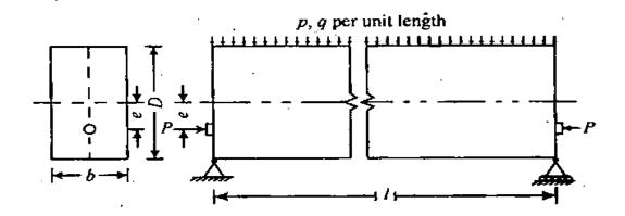
A simply supported high strength concrete beam of rectangular cross-section  $(b \times D)$ , shown in the above figure, supports uniformly distributed dead and live loads of intensities p and q per unit length respectively. The beam is prestressed by a straight tendon carrying a prestressing force P at an eccentricity e. Show clearly and neatly the stress distributions, through the beam depth, due to eccentric prestressing, dead and live loads at a cross-section where maximum stresses occur. 15
