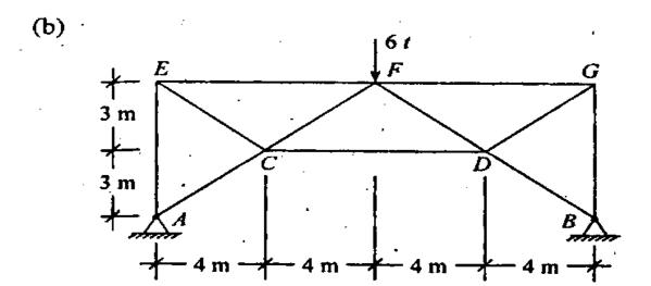
All the members of steel truss shown in the above figure are pin-jointed and have same area of cross-section.
