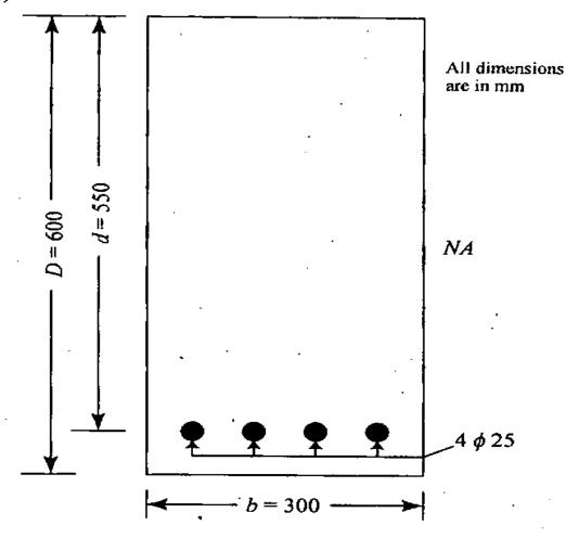
A reinforced concrete beam of rectangular cross-section (600 mm  $\times$  300 mm) is shown in the above figure. Assume M20 grade concrete and  $F_e$  415 grade steel. Permissible compressive stress of concrete in bending  $\sigma_{cbc} = 7.0$  MPa for M20 concrete.
