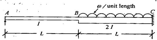
A stepped beam ABC, simply supported at A and fixed at C as shown in the above figure carries a uniformly distributed load of intensity '\omega' per unit length over BC. Determine the vertical reaction at A using moment area or energy method.
