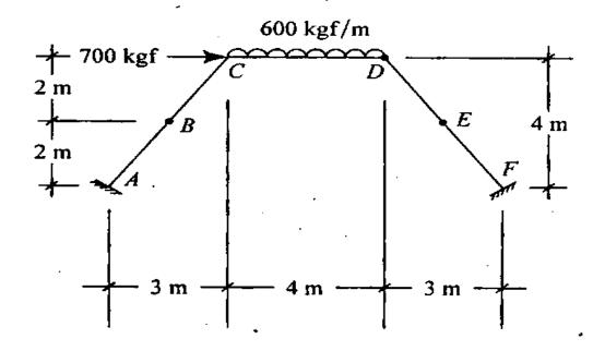
A portal frame ABCDEF with inclined legs has hinges at B, D and E as shown in the above figure. Joint at C is monolithic. Supports at A and F are fixed. Calculate all components of reactions.
