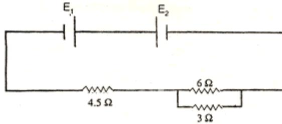
Calculate the value of current flowing through the resistance of  $3\Omega$ .
