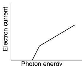
Sol: The electron current occurs above the threshold voltage. Initially the current rises steeply and then slowly attains saturation.
