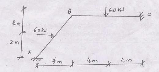
Analyse the beam shown in figure by column Analogy method and draw SFD & BMD. 10
