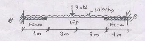
(b) For the non prismatic beam element shown in **figure**, calculate ke stiffness coefficients 10  $k_{11}$  and  $k_{21}$ . Also calculate COF from B to A.
