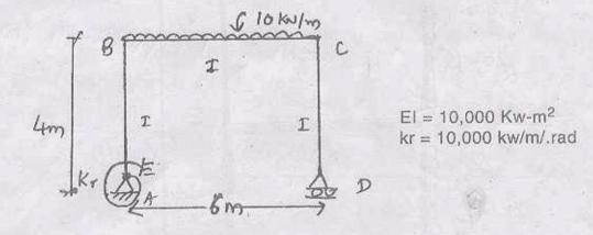
2. Analyse the frame shown in figure by elastic centre method and draw SFD, BMD.
