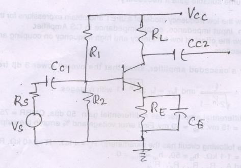
(b) For the amplifier shown below, it is desired to haul tower 3dβ frequency of not more than 20 Hz. If  $h_{ie} = 1.1 \text{ k}\Omega$ .  $h_{fe} = 120$ ,  $R_s = 100 \Omega$ . What is the value of C<sub>C</sub> required ?
