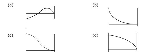
46. A cantilever beam has the square cross section of  $10 \text{ mm} \times 10 \text{ mm}$ . It carries a transverse load of 10 N. considering only the bottom fibres of the beam, the correct representation of the longitudinal variation of the bending stress is
