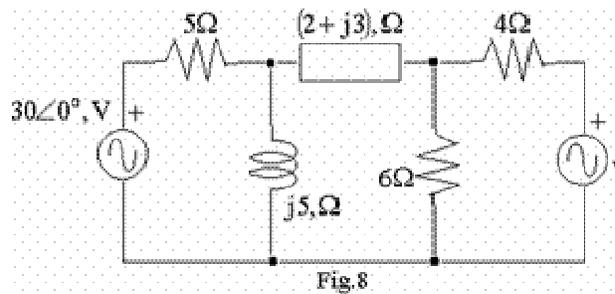
b. Find  $v_x$  in the network of Fig.8, if the current through  $(2 + j3)$  element is zero. (8)
