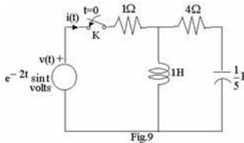
b. Find the transform current  $I(s)$  drawn by the source shown in Fig.9 when switch  $K$  is closed at time  $t = 0$ . Assume zero initial conditions. (8)
