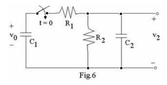
Q.5 In the network shown in Fig.6 below,  $C_1 = C_2 = 1F$  and  $R_1 = R_2 = 1\Omega$ . The capacitor  $C_1$  is charged to  $V_0 = 1V$  and connected across the  $R_1 - R_2 - C_2$  network at t = 0.  $C_2$  is initially uncharged. Find an expression for  $v_2(t)$ . . (14)
