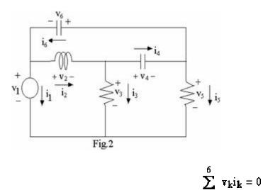
Q.2 a. In the circuit shown in Fig.2 below, it is claimed that k=1. Prove OR disprove. (7)
