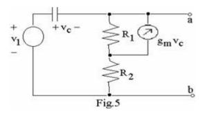
b. Determine the equivalent Norton network at the terminals a and b of the circuit shown in Fig.5 below. (7)
