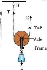
The load L is balanced by the tension in two segments of the string and the effort E balances the tension T at the free end, so
