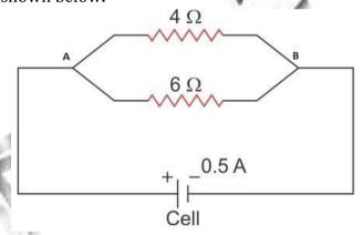
ii. In parallel combination of resistors potential difference across each resistor is same as the potential difference across the terminals of the battery.
